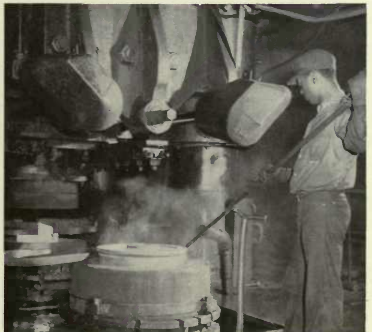
One of the stages in the forging of a railroad wheel, another specialty product of U. S. Steel for the carriers.
